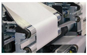
PlasmaMAX<sup>™</sup> creates functional thin-film layers of metal oxides, nitrides, oxynitrides, and polymers on almost any substrate. The substrate form can be a rigid panel or a flexible web, while the substrate material can be glass, polymer, or metal. PlasmaMAX<sup>™</sup> can even coat conductive and magnetic substrates (e.g., steel) because it does not require the use of costly magnets or high frequency power supplies which are typically required in other coating systems.
