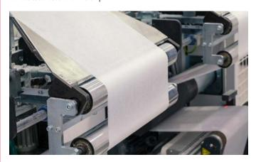
PlasmaMAX<sup>TM</sup> creates functional thin-film layers of metal oxides, nitrides, oxy-nitrides, and polymers on almost any substrate. The substrate form can be a rigid panel or a flexible web, while the substrate material can be glass, polymer, or metal. PlasmaMAX<sup>TM</sup> can even coat conductive and magnetic substrates (e.g., steel) because it does not require the use of costly magnets or high frequency power supplies which are typically required in other coating systems.
