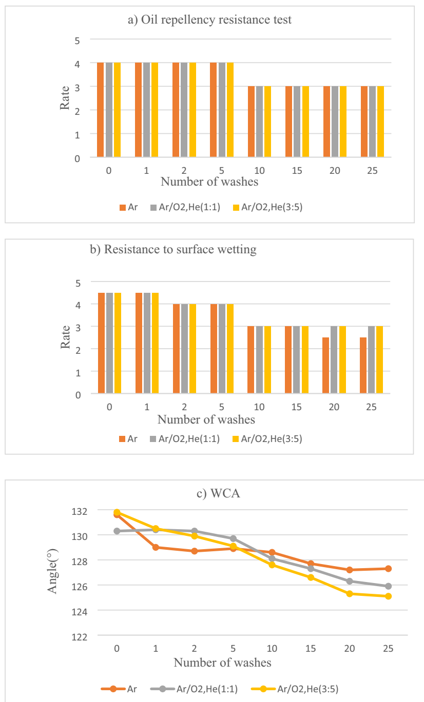
Fig. 3. Effect of gas mixture (a) drop test, (b) spray test, (c) WCA.
